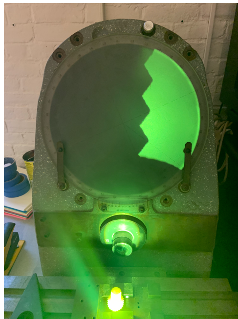
the view inside: screw threads being examined
