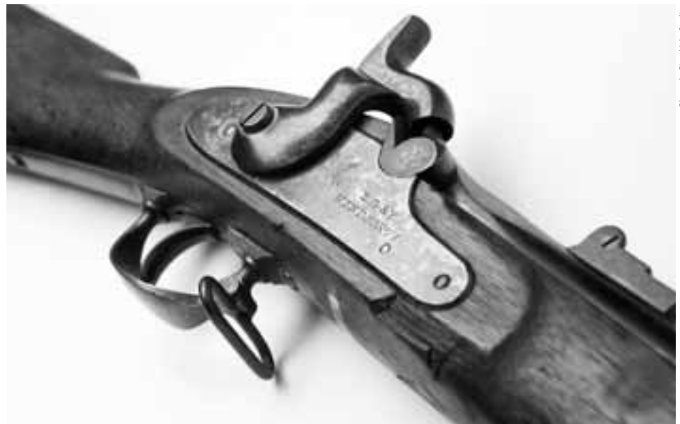
Special Model 1861 rifle, made by Lamson, Goodnow & Yale, Windsor VT, circa 1863 This was the most common firearm for Union soldiers with an effective range well over 200 yards, allowing it to be fired several times a minute. The Amoskeag Machine Company in Nashua, New Hampshire, was outfitted with Lamson machinery and also produced this model.
