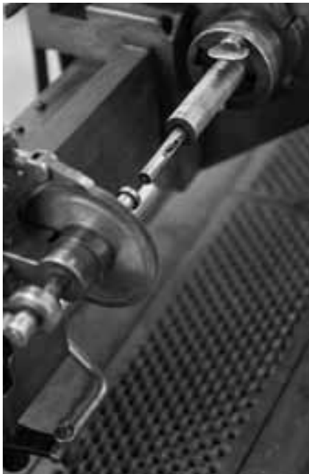
Rifling Machine Robbins & Lawrence, Windsor, Vermont, circa 1853 In the 1850s, machine designers, including those in Windsor, developed rifling machines for cutting the parallel spiral grooves inside the gun barrel so a bullet could be made to spin as it flies.
