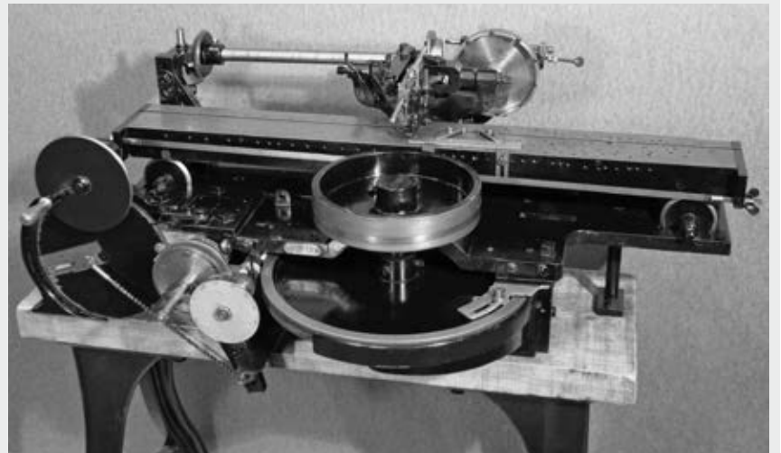
This 1850 linear dividing engine was used by Brown & Sharpe to cut the graduations on vernier calipers and machinist's rules. It is the first of its kind.
